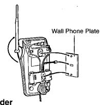
Connect the AC adaptor. Tuck the telephone line cord inside the wall mounting adaptor, then push it in the direction of the arrow.
