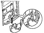
Connect the telephone line cord. Mount the unit, then slide down.
